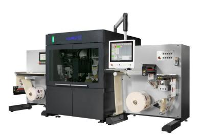
The standalone DM-Uniliner digital metallization unit from Kurz (Photo: Kurz)
